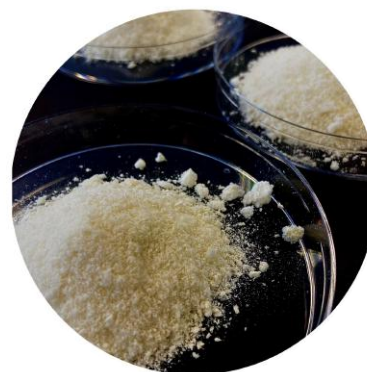
Fig. 17 Spray dryer enzyme powder obtained from 10m 3 fermentation broth
